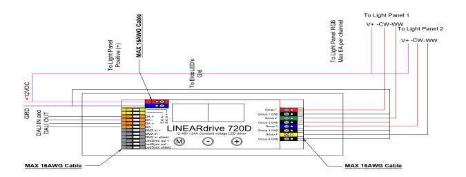
EldoLED configuration with linear dimming curve and white colour mode.
