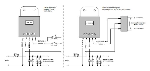
No direct load can be put onto the master dimmer. The master can only be used to control the slaves that have the load.
