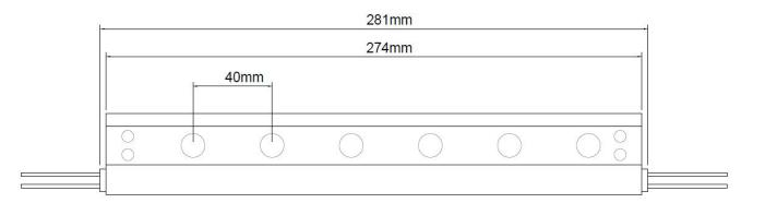
Maximum quantity in series: 15 modules. Connect further modules in parallel
